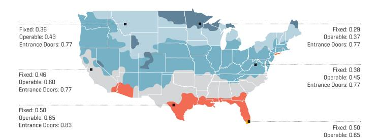
of the 2015 IBC outlines the locations where impact-resistant products are required. All exterior openings in wind-borne debris areas are required to be impact resistant in the 2015 IBC. Determination of wind-borne debris
